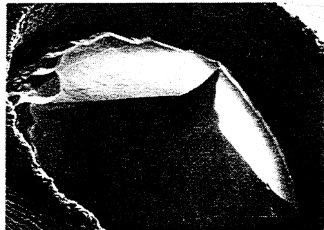
Figure 5. ES-423E Cathode after 10,000 hours in Philips EM-420 TEM at around 1750 K. Crystal almost completely gone. Heater structure unchanged.
